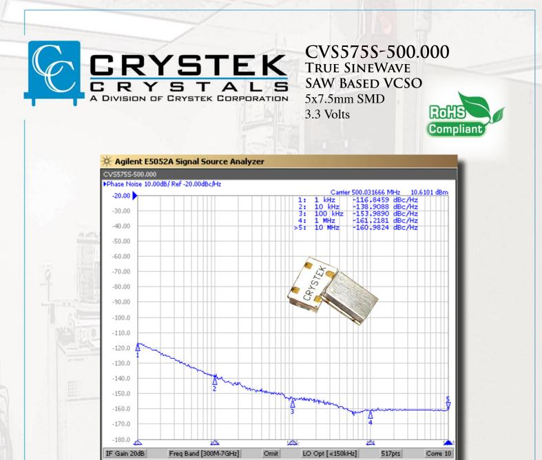
Model CVS575S-500 is a 500MHz voltage-controlled SAW (surface acoustic wave) oscillator (VCSO). SAW crystal technology provides low-noise and low-jitter performance with true sinewave output. Features include -135dBc/Hz phase noise at 10kHz offset, 3.3V input voltage, -20 to +70C operating temperature, and 5x7.5 mm SMT package. The oscillator has no sub-harmonic and the second harmonic is typically -14dBc.
